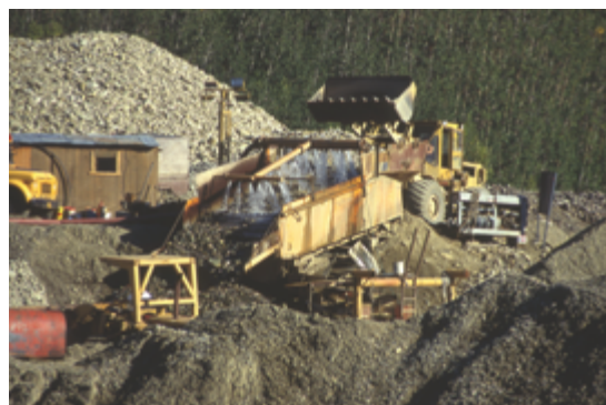
Fig. 13. Loading gravel into a small screening plant at a Klondike placer mine.
