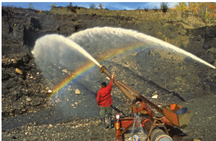
Fig. 12. Monitor pumps at a hydraulicking operation on Hester Creek cut into a thick cover of organic muck overlying gold-bearing gravels. The end of the rainbow is on mineralised Klondike Schist that is also washed out by the water jets.
